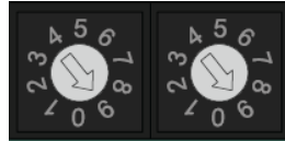
Example: Rotary Switch showing ID No. 99.
